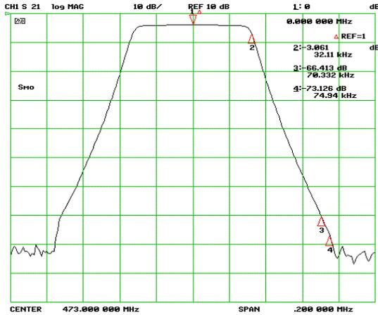
The filter's bandwidths & selectivity can be specified by the user in order to achieve very narrow filters windows, such as, for example, 70 dB rejection at 200 kHz offset for less than 13  $\mu$ sec, or 70 dB rejection at 90 kHz offset at the expense of 30  $\mu$ sec delay Typical digital filter frequency response, 30 micro-second Group-Delay, with 70 dB ACR @ 75 kHz offset. (Other Configurations are available, user field upgradeable).
