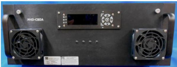
The CTI MARK-IV DIGITAL NARROWBAND SIGNAL BOOSTER, integrates two sets of front-end programmable narrowband filters with multi-carrier power amplifiers, to deliver a Bi-Directional Narrowband Signal Booster. The individual AGC per channel feature essentially reduces the uplink near-far concern prevalent in many Public Safety broadband DAS systems.
