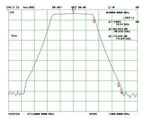
The filter's bandwidths & selectivity can be specified by the user in order to achieve very narrow filters windows, such as, for example, 70 dB rejection at 200 kHz offset for less than 13  $\mu sec$ , or 70 dB rejection at 90 kHz offset at the expense of 30  $\mu sec$  delay Typical digital filter frequency response, 30 micro-second Group-Delay, with 70 dB ACR @ 75 kHz offset. (Other Configurations are available, user field upgradeable).
