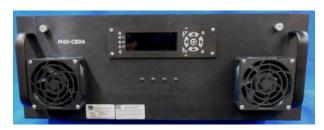
The CTI MARK-IV DIGITAL NARROWBAND SIGNAL BOOSTER, integrates two sets of front-end programmable narrowband filters with multi-carrier power amplifiers, to deliver a Bi-Directional Narrowband Signal Booster. The individual AGC per channel feature essentially reduces the uplink near-far concern prevalent in many Public Safety broadband DAS systems.
